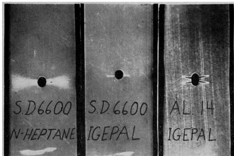
Fig. 4. Photograph of samples on the verge of fracture under stress cracking conditions: left , a linear polymer with n -heptane as the stress cracking agent, middle , a linear polymer, Super Dylan 6600, with Igepal; right , a branched polymer, Alathon 14, in Igepal.
